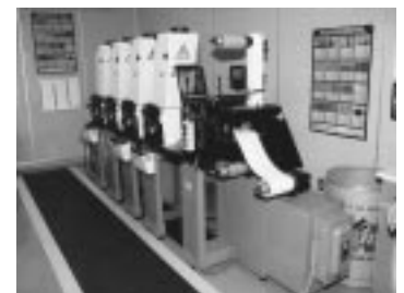
The Comco 7" web press in the Penn College flexography lab. Photo by Richard Rutledge.
