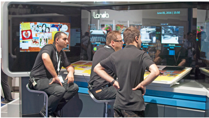
Press Operators monitoring the progress of printing from the Landa Operator Cockpit. This control center features an inspection table, touch screen controls, counter, and utility drawers.
