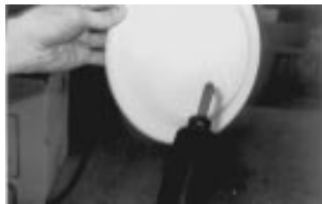
Don't let the flame treating scare you away from this project. Passing the flame from a propane torch quickly across the surface removes the manufacturing oils.
