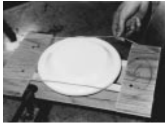
The flyer is quickly mounted onto the fixture with two rubberbands to hold the flyer in place during printing.
