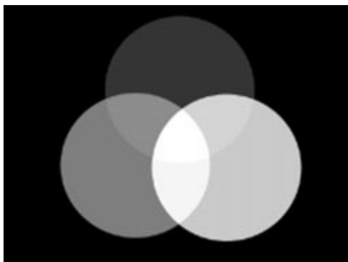
Figure 3c. The additive color mixing principle.
