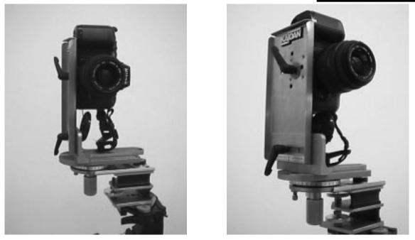
Figure 4. Below is a tripod head specifically designed for creating QTVR Panoramas. The camera is suspended exactly over the point of rotation. The camera is rotated and 15-30 separate overlapping pictures are taken to create one panorama.
