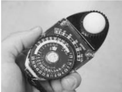
Figure 12: A simple hand held light meter can be used to measure the lighting ratio between highlight and shadow.
