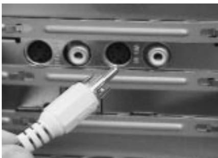
*Figure 6: These are the video input/output ports of a video capture card on the back of a computer. A video capture or digitizing card takes input from a standard analog video source and converts it to digital data.*
